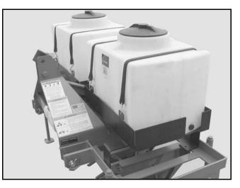
Figure 8. Water Tanks Installed
